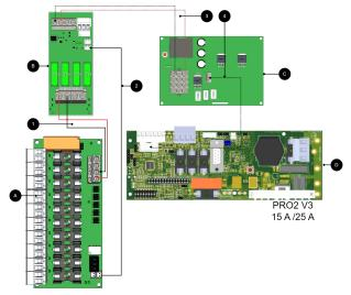
+ and - from load on motherboard are connected to + and - on the option board.
