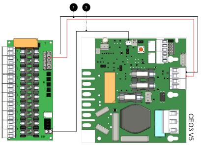
+ and - from load on motherboard are connected to + and - on the option board.
