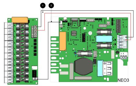
+ and - from load on motherboard are connected to + and - on the option board.
