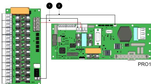
+ and - from load on motherboard are connected to + and - on the option card.
