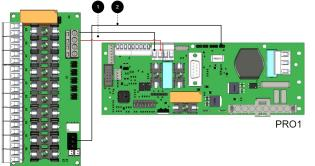
Older cards<sup>1</sup> which lacks a JST contact, then the alarm is connected via relay switching. P3:1-3
