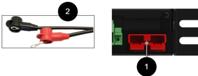
Use the included cabling to connect the batteries. Be careful not to short the terminals of the batteries. First connect wiring in batteries, (2). Cabling must have rubber pole protection that covers the battery pole. Then connect battery connector to the battery backup, (1).
