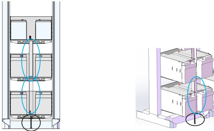
Support between battery shelves is included in Battery shelf 24V L and must be mounted. Support is not needed for Battery Shelf 24V M.
