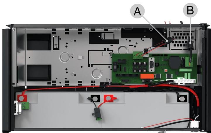
A ferrite on EN54 shall be threaded one pass on load cables (A).
