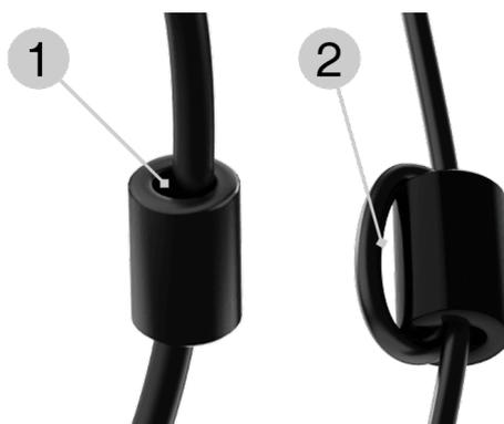
A "pass" is how many times the cable passes through the ferrite.
