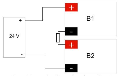
Connect the terminals correctly so that you do not damage the equipment.
