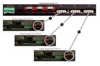
Connect Redundancy panel 1U with Power supply 24V 15A 1U
