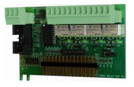
With 4 pcs. relay outputs for systems supplied with PRO2 v3 motherboards.
