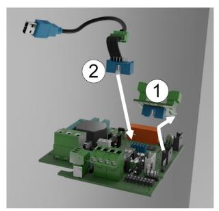
If when the card is removed an alarm can be given, then the connection to the power supply has been broken. Cards on the connector may vary.
