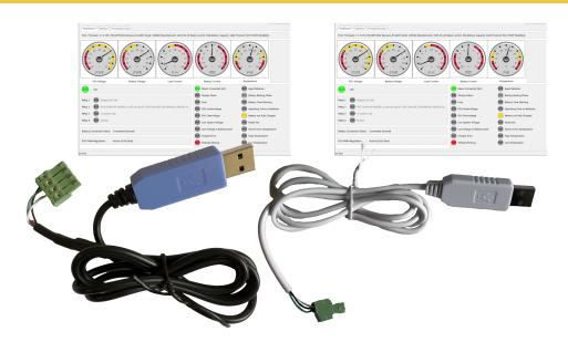
PowerWatch is available in two variants: PowerWatch (blue USB) and PowerWatch RACK (white USB).
