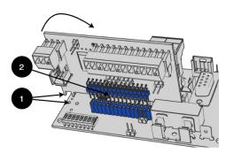
Lift the card to remove it and reseat it after the device is updated with Power-Watch.
