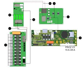
+ and - from load on motherboard are connected to + and - on the option board.
