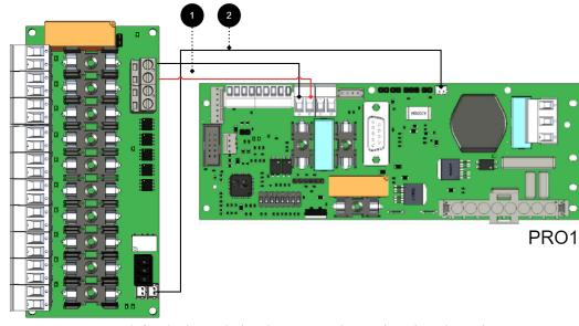
+ and - from load on motherboard are connected to + and - on the option card.
