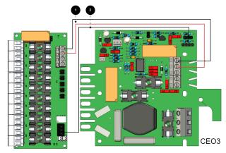
+ and - from load on motherboard are connected to + and - on the option board.
