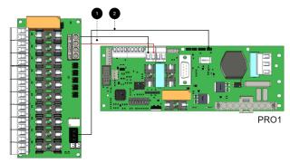
Older cards<sup>1</sup> which lacks a JST contact, then the alarm is connected via relay switching. P3:1-3
