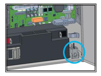
Connecting Battery Shelf 24V M / Battery Shelf 24V L for battery backup
