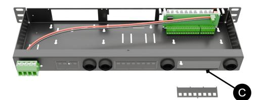
Cut off the plate with which the knock-out (C) is stuck.
