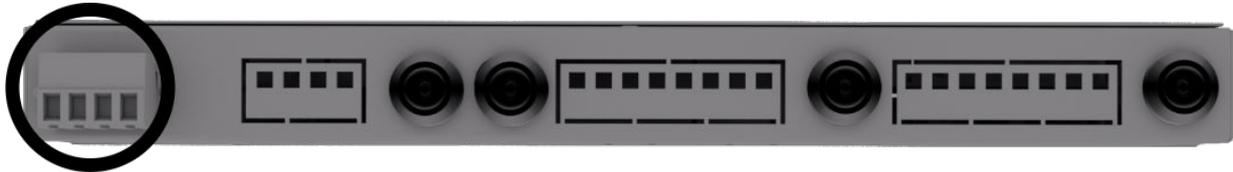
Switching on 24V takes place on the back, via the jackable terminal.
