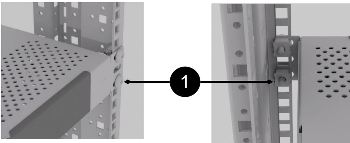
The unit is a height unit (44 mm) high, and should be mounted in 19" racks with two screws on each side (1).
