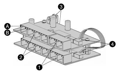
Two cards are connected with cable on 4, or a patch cable between 1 on each card.
