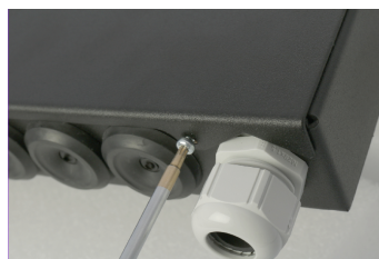
5. Skruva fast locket, (2skruv).
