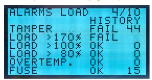
Alarm from tamper contact, load, temperature and fuse
