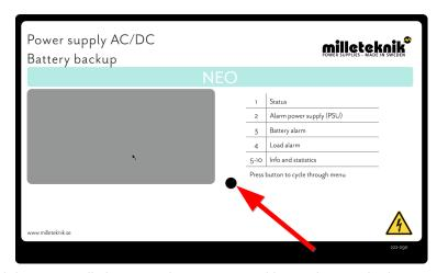
The push button scrolls between the screens and is used to set the battery capacity.
